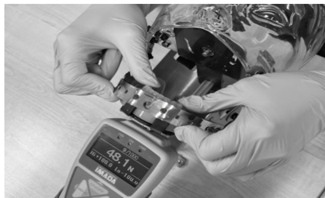
Figure 2. The instructed method for applying force to the FD Participants were instructed to place their thumbs around the second premolar of the FD and apply force with both hands by clamping the other four fingers between the metal frames corresponding to the lower margin of the mandible
