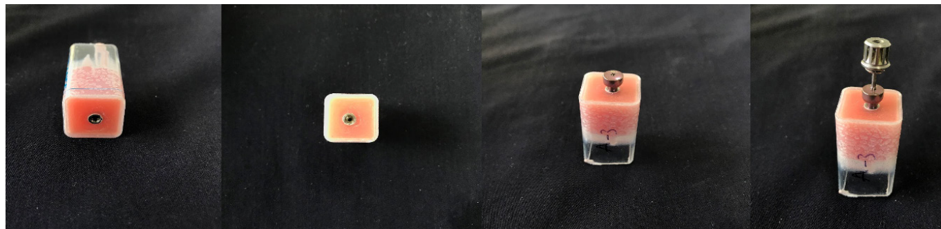
Figure 1. A setup was prepared with an implant screw embedded in cold acrylic to manually torque the healing cap.
